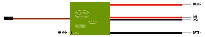
JUMPER ON = BEC SELECTED JUMPER OFF = BEC DISCONNECTED
